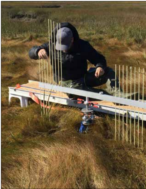
Taking saltmarsh surface readings with a Sediment Elevation Table.
